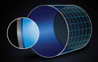
This Blue Diamond<sup>®</sup> technology provides twice the corrosion resistance compared to industry standards and increases the life span of the tank.
